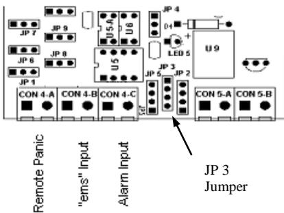
**JP3 for CON 5-A Output Monitoring Circuit**
